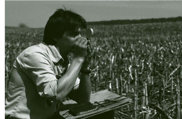
Figure 3.1.9 Slope Grade Measurement Using a Clinometer
