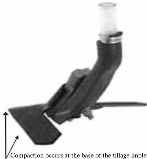
Figure 2. Soil compaction occurs at the base of the cultivator shovel or base of other types of tillage equipment. The level of compaction is increased as soil moisture content is increased or when the soil clay and silt content is higher.
