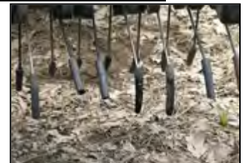
Machine with rubber finger tips for removing trash from overwintered strawberries
