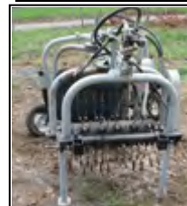
Machine with rubber finger tips for removing trash from overwintered strawberries
