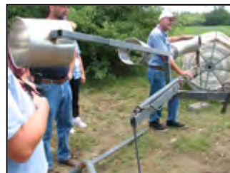
Equipment to help roll row cover onto reels
