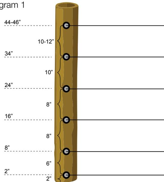
Wire spacing and height outlined here is critical in preventing low spots in the fence or large gaps between electric wires.
