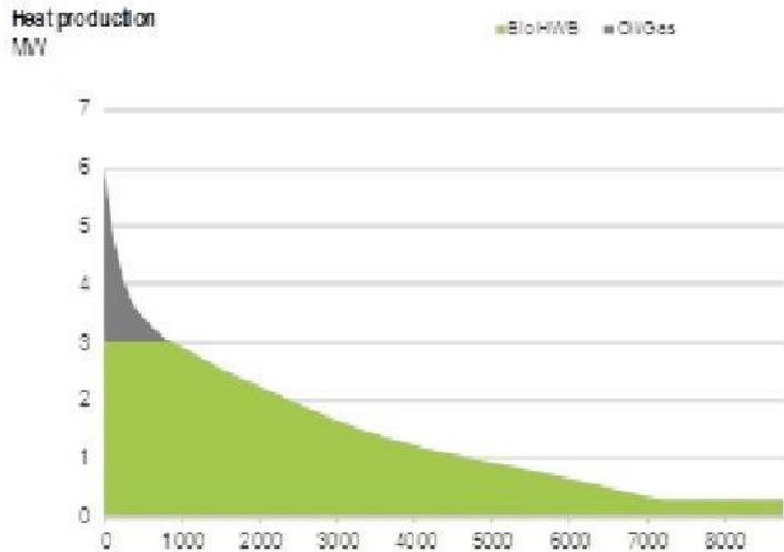
Figure 15: Typical heat load duration curve. Green is met by biomass, blue by heating oil or natural gas. Source: Natural Resources Canada and FVB Energy via Canadian District Energy Association Biomass for District Heating module.
