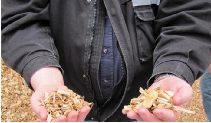
**Figure 8: Different kinds of chip. To the left the smaller chip meets the European 'G30' standard and to the right the 'G50' standard.**
