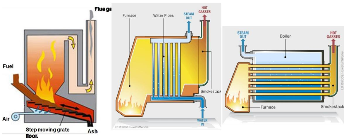
Figure 13: Left – grate furnace, centre – fire tube boiler (up to ~25MW), and right – water tube boiler (from ~2MW +). Furnace and boiler components combine to form what is normally referred to as a “boiler”.
