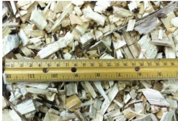
Figure 7: wood chip dimensions. Source: FPInnovations
