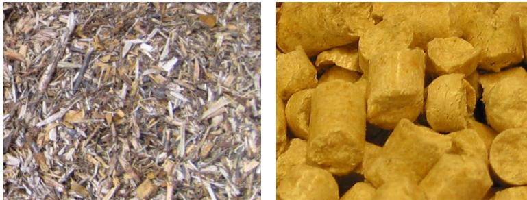
Figure 5: Wood chip and wood pellet. Source: FPInnovations
