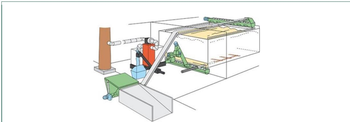
Figure 12: Energy centre for a 2 MW wood fuel boiler, showing wood fuel delivery area, fuel store, fuel transfer / feed mechanisms, ash handling system, and flue. Source: Natural Resources Canada and FVB Energy via Canadian District Energy Association *Biomass for District Heating* module.
