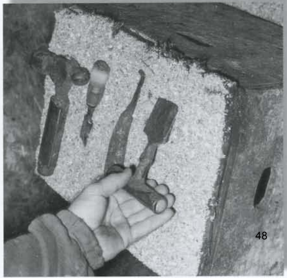
Tools used for trimming feet include (bottom to top) a 2-inch chisel with T-bar; hoof knife; 1-inch chisel and hammer.
