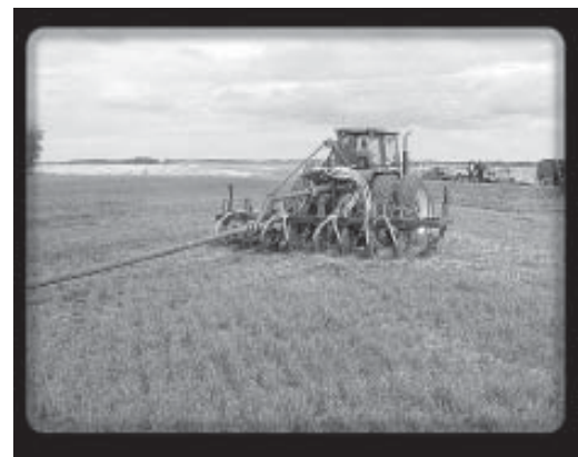
Post emergent injection with a modified aerway system
