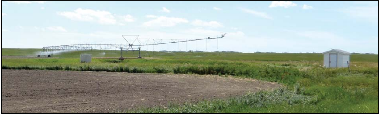
Figure 5.18. Pivot irrigation system at the Battersea Drain Field showing the corner arm nozzles turned off as the pivot passed over the runoff sensitive area of the northeast corner on July 16, 2010.
