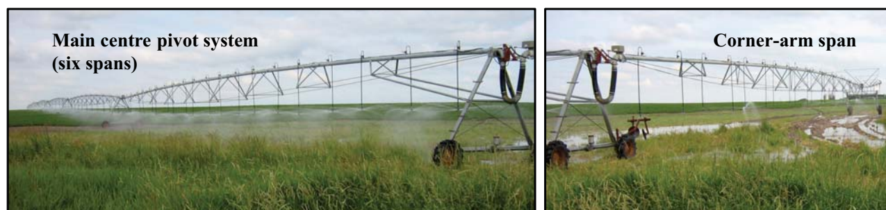
Figure 5.3. The centre pivot irrigation system showing the main system of six spans (left) and the corner-arm span (right) at the Battersea Drain Field.
