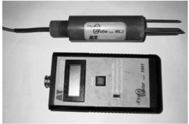
Figure 3. Theta probe by Delta-T technologies.
