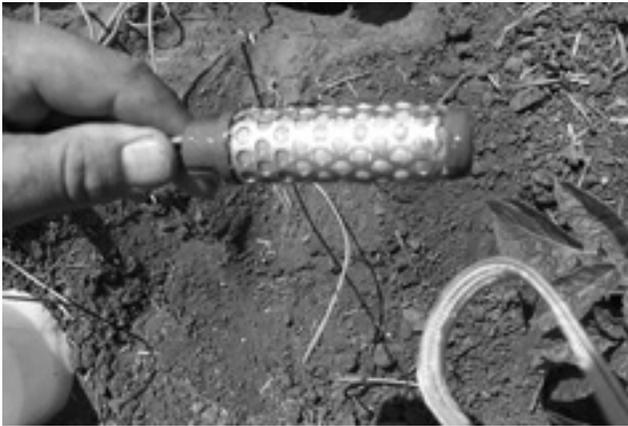
Figure 4. Watermark sensor by Irrometer.
