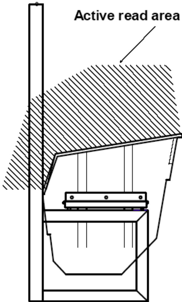
**Antenna in each feed bunk emits an electromagnetic field which activates the transponder tag**
