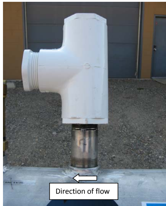
Figure 1. Originally designed LOPAC flow monitor equipped with non resettable counter only (at left) and Model LHE2 with additional PVC housing and data logger (at right).
