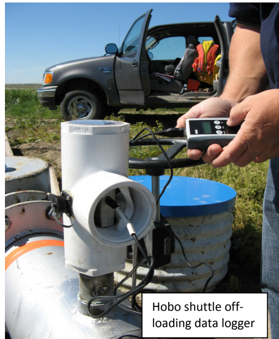
Figure 2. Time counter installed in top of the PVC housing displays time of flow in hours and minutes (at left) and accessing data logger in horizontal portion of PVC housing (at right).
