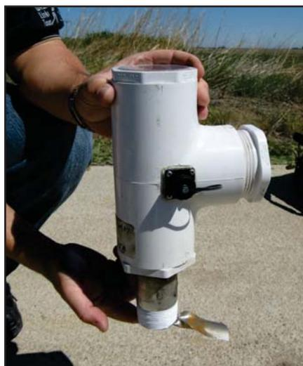
**Orient with paddle angled with direction of flow**
