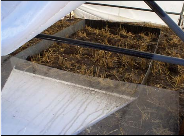
Fig. 5. (above) Runoff frame, collection tray, and plexiglass cover during rainfall simulation.
