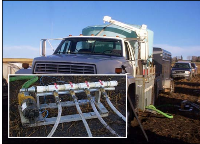
Fig. 4. Water truck, pump, and header system.
