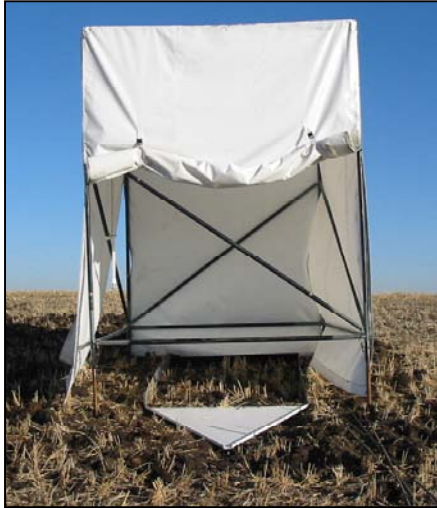
Fig. 3. Rainfall simulator, runoff frame, and collection tray.
