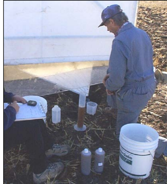
Fig. 5. (above) Runoff frame, collection tray, and plexiglass cover during rainfall simulation.
