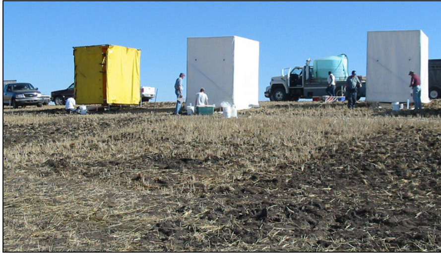
Fig. 2. Three of the four rainfall simulators used simultaneously.
