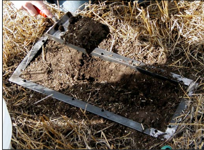
Fig. 1. Frame-excitation method of soil sampling.
