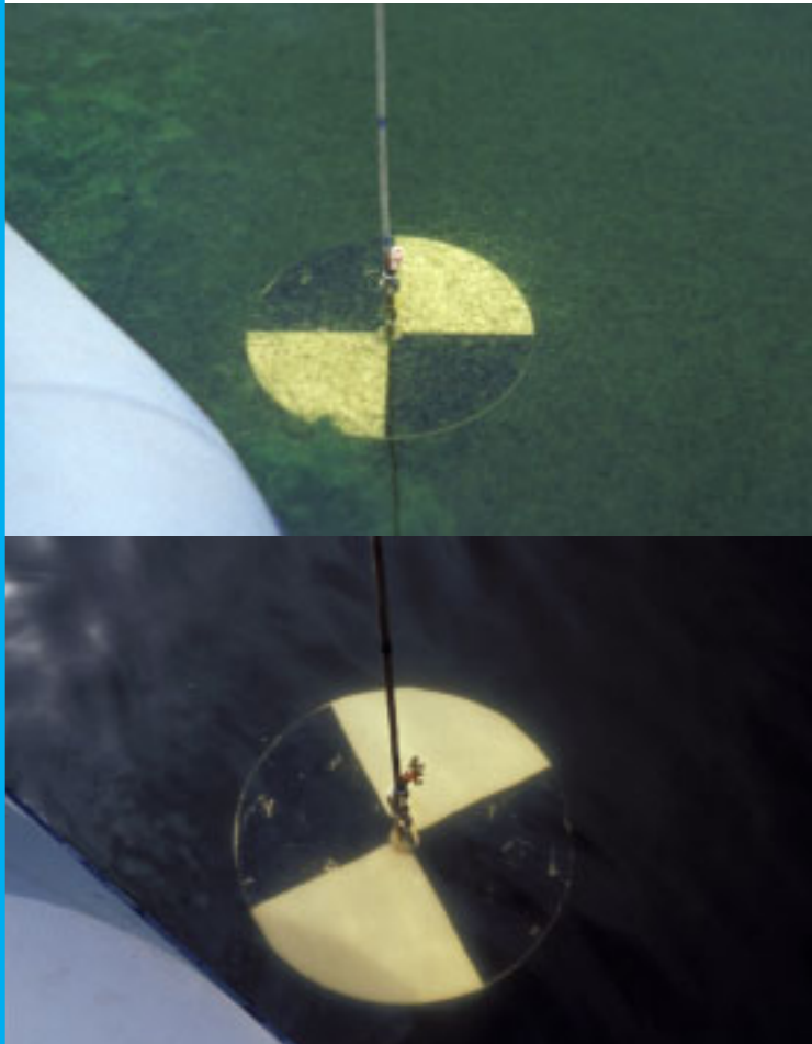
A secchi disk showing dugout water before and after a successful treatment of one type of cyanobacteria
