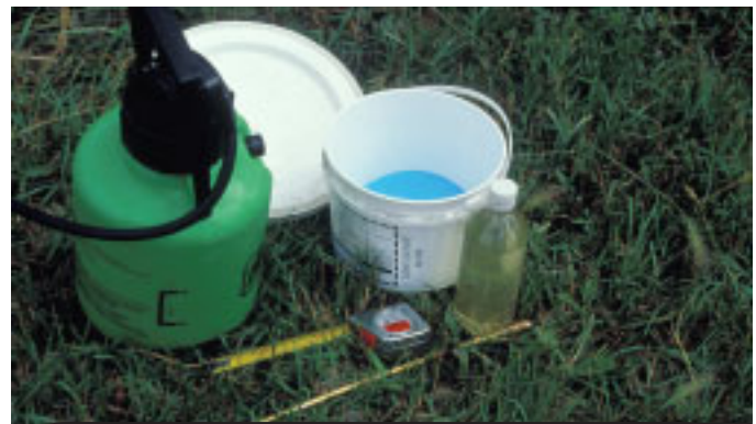
A 10 L hand pump spray applicator is ideal for small dugouts
