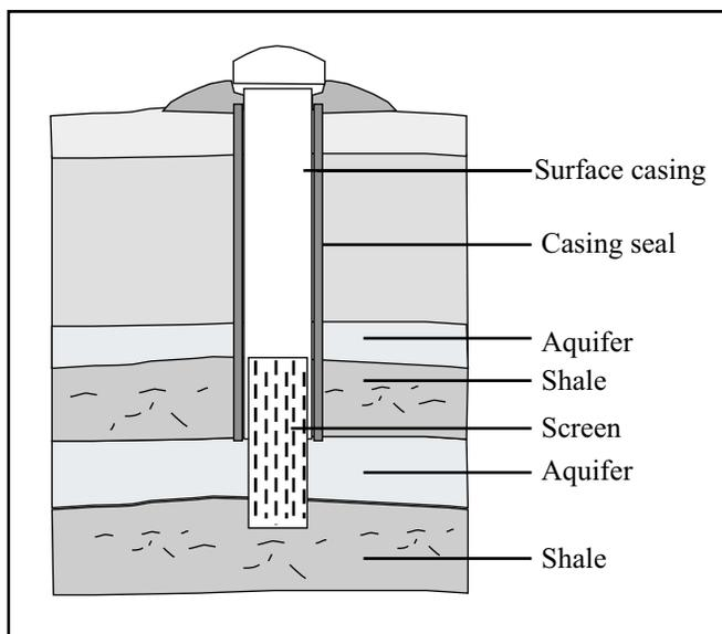
**Figure 2. Properly screened well.**
