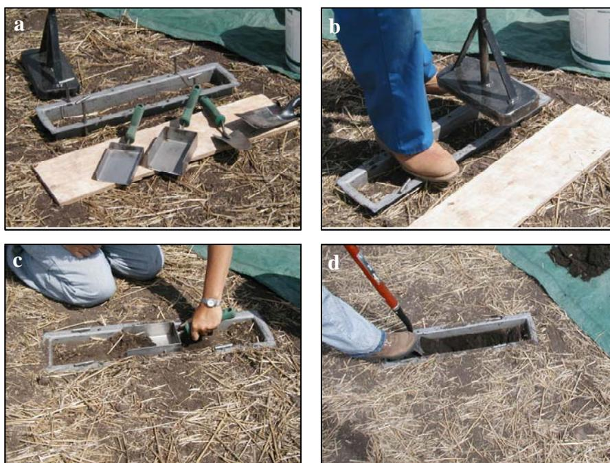
**Fig. 1.** Frame-excitation sampling technique showing (a) tools, (b) frame installation, (c) removal of the top two layers (0 to 2.5 cm and 2.5 to 5 cm) with scoops, and (d) removal of the third layer (5 to 15 cm) with a shovel.
