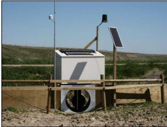
**Fig. 4.** Instrumentation at the LLB site showing the plywood-reinforced berm and flume.
