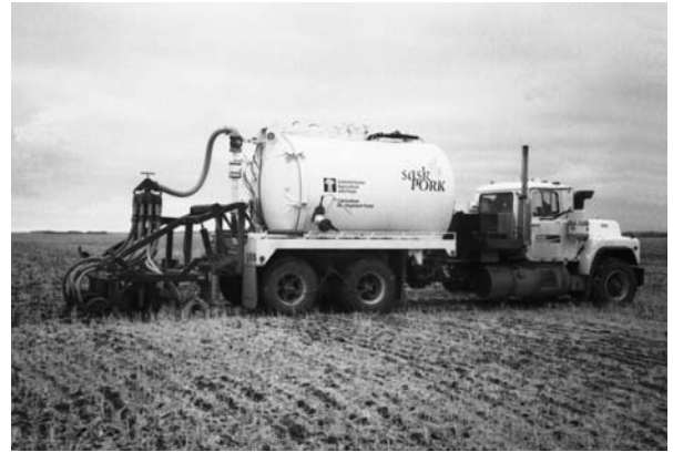
Figure 8. PAMI manure research truck fitted with low disturbance disc openers for liquid manure injection Source: PAMI, 2002.
