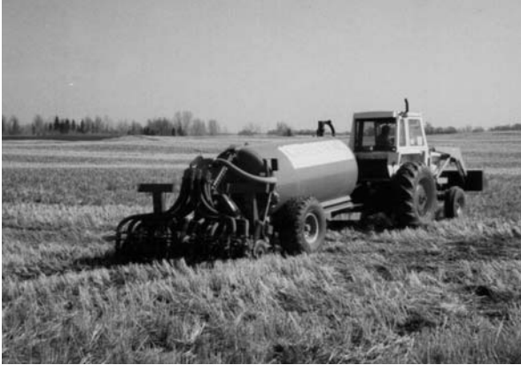
Figure 7. Liquid manure injection system using a tool bar mounted on a tanker Source: PAMI, 2003 (Carol Jackson person.comm.).
