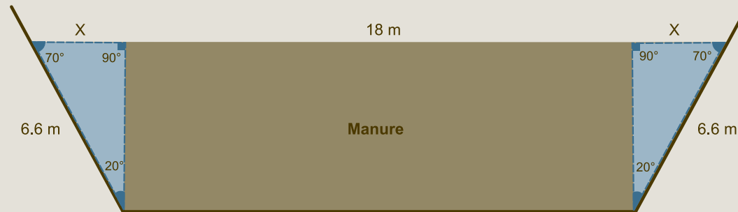
Figure 4.1.15 Dimensions for Calculating the Width and Length of the Surface of the Manure in Storage
