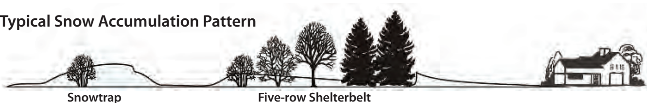
Figure 48: Typical snow trapping with shelterbelts and use of shrub row to enhance snow trapping. Figure courtesy of PFRA
