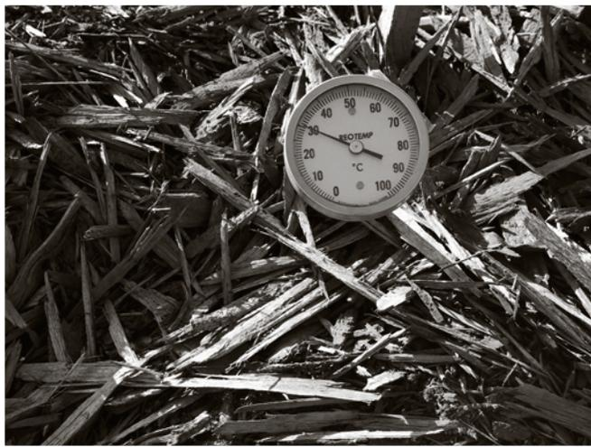
The temperature can be measured with a 1 metre (3 foot) long dial temperature probe.
