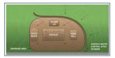
Illustration of location of control ditch or berm.
