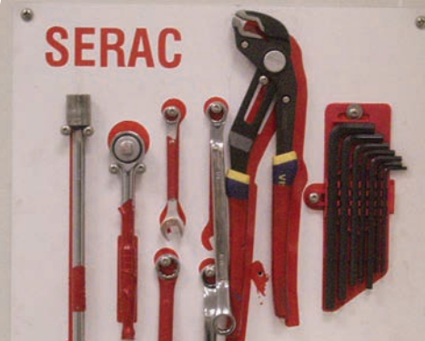
Shadow board organized by shape and colour.
