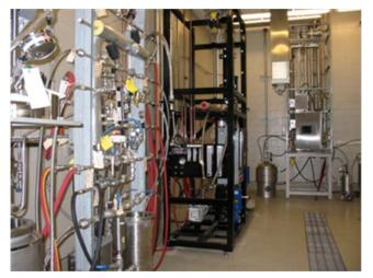
Bio-Industrial Opportunities Branch is one of several stakeholders involved in the operation of a \$2 million polyol pilot plant located at Agri-Food Discovery Place in Edmonton. The plant enables focused research into the ozonolysis and hydrogenation processes required to turn canola oil into a diverse class of chemicals known as polyols, as well as industrial acids.
