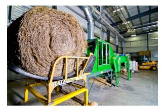
Purchased in 2009 at a cost of \$4.5 million, ABDC's Belgian-made Van Dommele unit can process one tonne of hemp or flax straw per hour into various grades of fibres for commercial biomaterials. Considered to be the largest publicly available fibre processing line in the world, this facility and the expertise that goes with it are attracting considerable commercial interest to Alberta.
