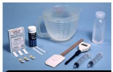
Beaker tests are required to determine the chemical dosage and provide an indication of the expected results
