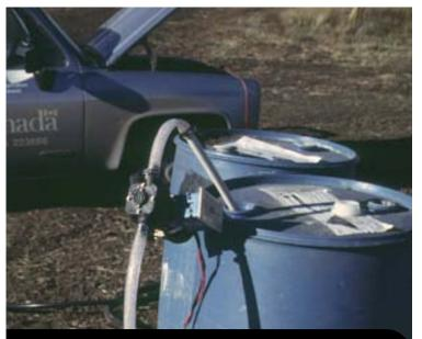
The coagulant chemical is pumped from the plastic barrel. Rinsing of the pump is critical to prevent impellor corrosion
