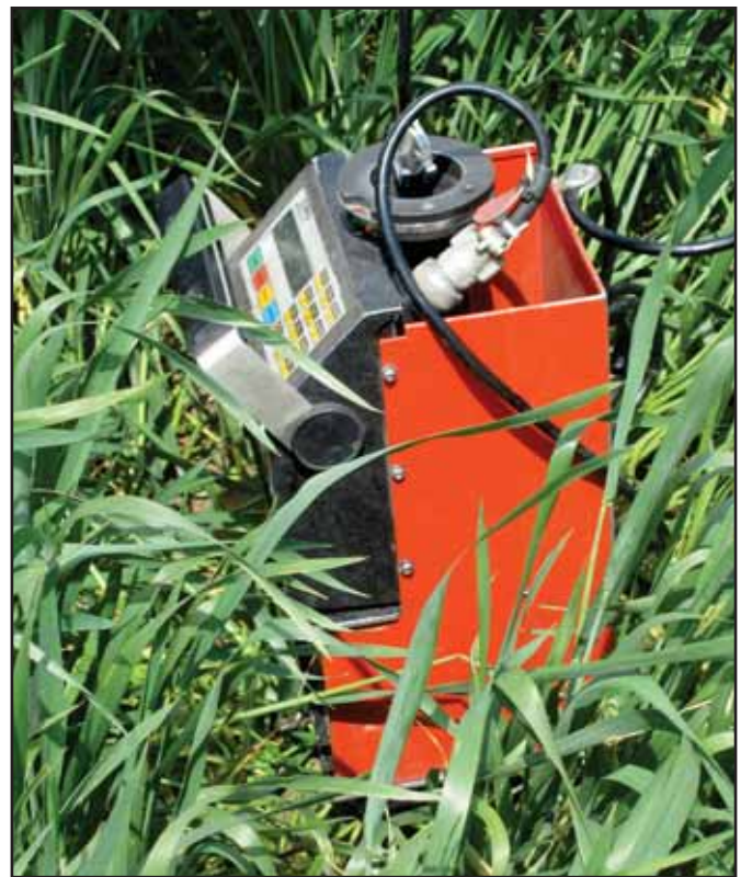
Figure 5. Campbell Pacific Nuclear International Inc. neutron moisture meter.
