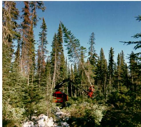
**Figure 31. Feller Buncher Harvesting**
