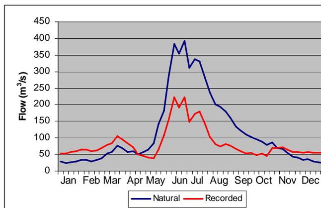
**Figure 3.7 Mean Monthly Recorded and Naturalized Flow for Bow River Near the Mouth, 1992–2001**
