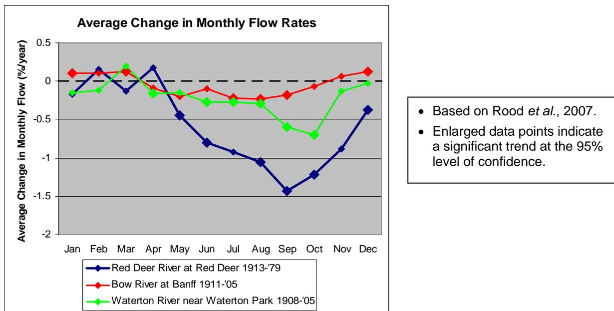
**Figure 3.11 Percent Change Rates Based on Slope of the Regression Equation for Monthly Flow Versus Year**
