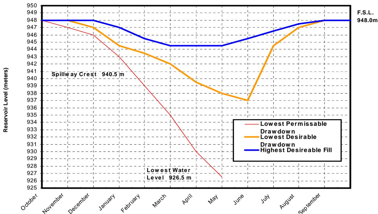
**Figure 6.1 Gleniffer Reservoir Operating Rule Curves**
