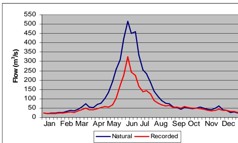
**Figure 3.8 Mean Monthly Recorded and Naturalized Flow for Oldman River Near the Mouth, 1992– 2001**
