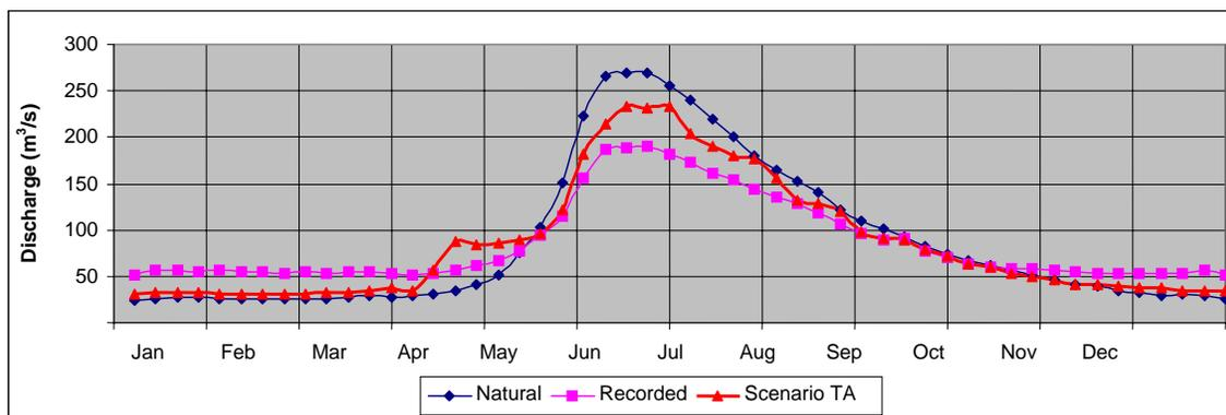
**Figure 6.7 Scenario TA Simulated Mean Weekly Flow Compared with Natural and Recorded Flows at Calgary**
