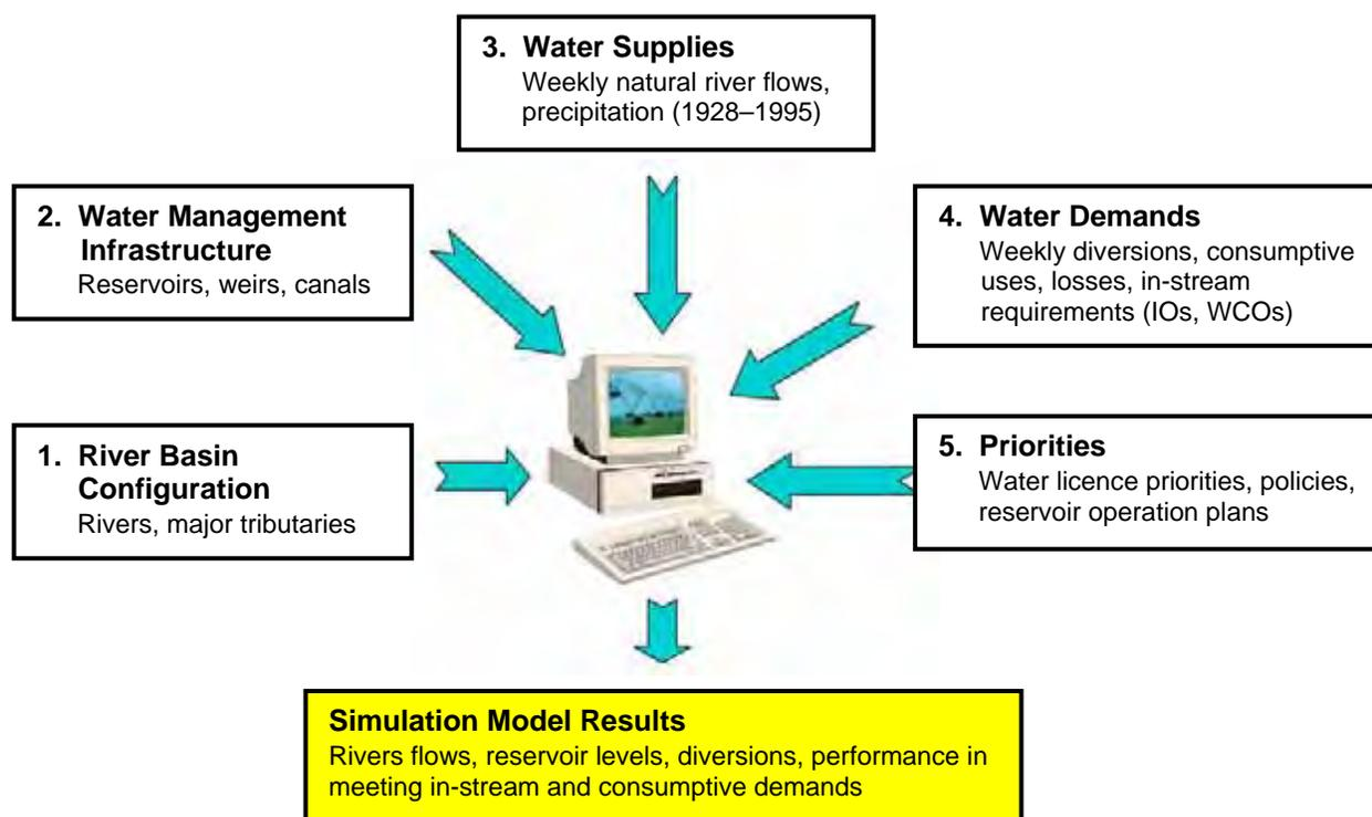
**Figure 5.1 Input Data Required for Simulation Modelling in this Study**
