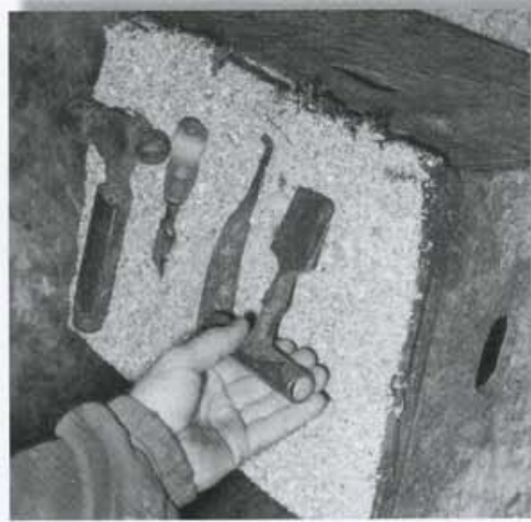
Tools used for trimming feet include (bottom to top) a 2-inch chisel with T-bar; hoof knife; 1-inch chisel and hammer.
