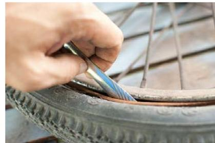
5. Take off the wheel and tube completely and inspect the tube for a puncture. Determine if the tube can be patched using a **patch kit** or if it must be replaced. Once you've either patched the old tube or are using a new tube, you're ready to replace the tire.
