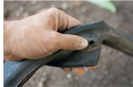
6. Partially inflate the tube and ease it into the tire, making sure the valve lines up properly. Make sure no part of the tube sticks out of the tire.
