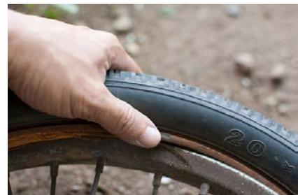
8. Before you inflate the tube, use your thumbs to ease the tire from the rim all around, looking in to ensure the tire isn't pinching any area of the tube against the rim. If it is, and you inflate the tube, it could pop and you'll have to repeat the whole process with a new tube.
