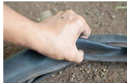
7. Starting at the edge closest to the valve, use your thumbs to work the other side of the tire over the rim and into the well. You may need to use your tire lever to get the tire back into the proper place.
