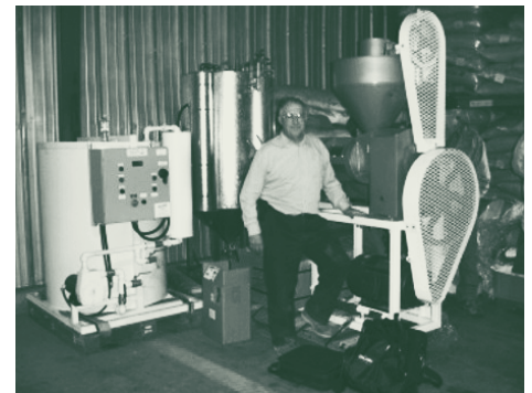
CPCS’s seed press, reactor tank and preheater tank (right to left) being examined by Danette engineer.
