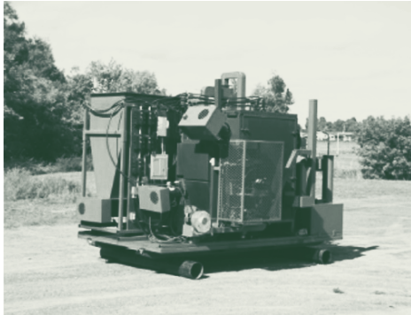
Pyrolysis system for converting chicken manure into a bioliquid
