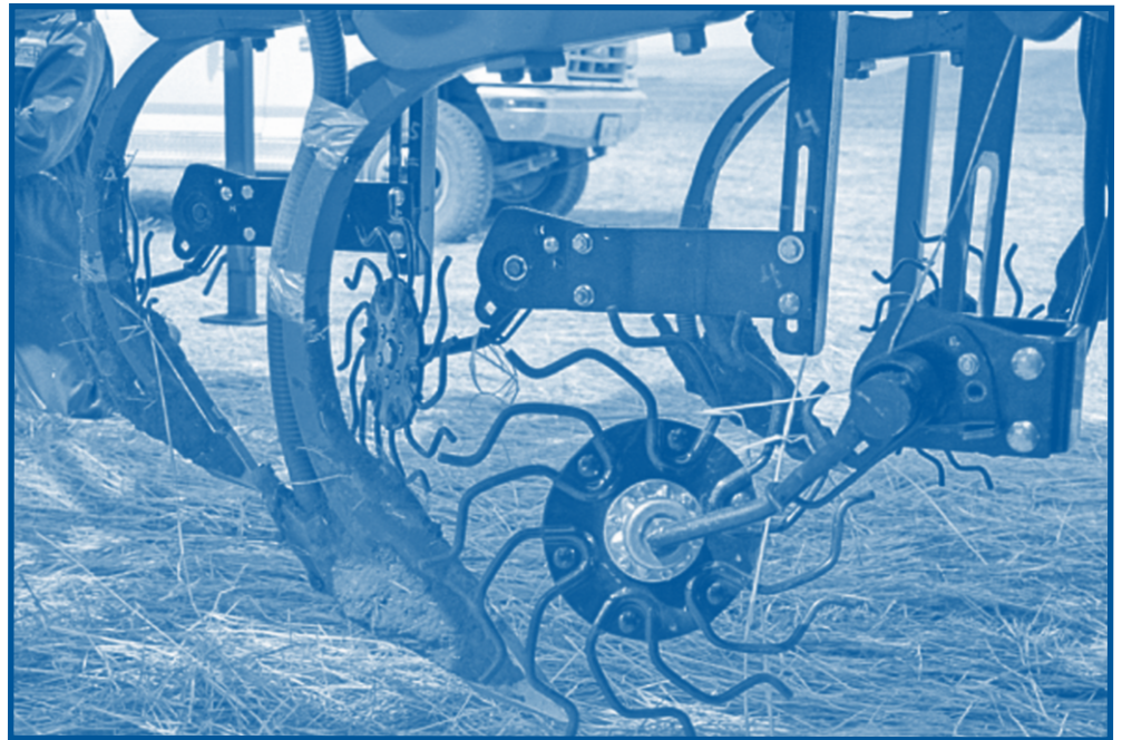
Residue managers have become a key field of research at the AgTech Centre. Pictured is a Terra-Tine row cleaner by Great Plains Manufacturing.
