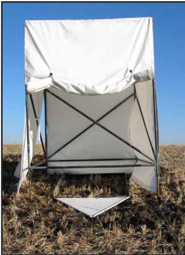
Figure 4.5. Rainfall simulator, runoff frame and collection tray used at the three field sites.
