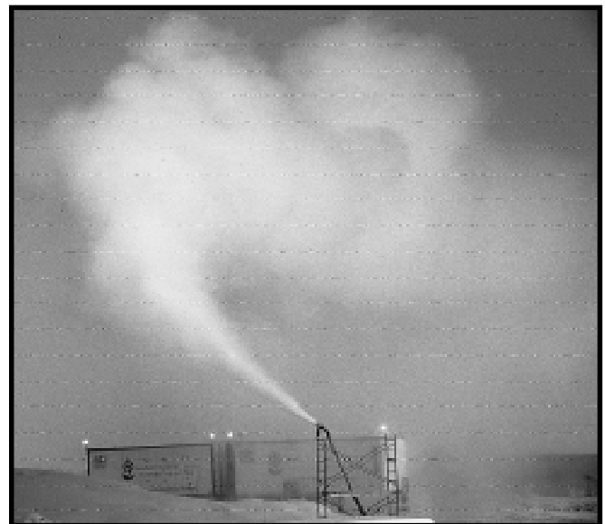
Snowfluent's mobile plant in operation at the Giebelhaus hog farm near Vegreville. The treatment process appears to fit economically into a conventional liquid manure management system without significant changes to equipment or layout.
