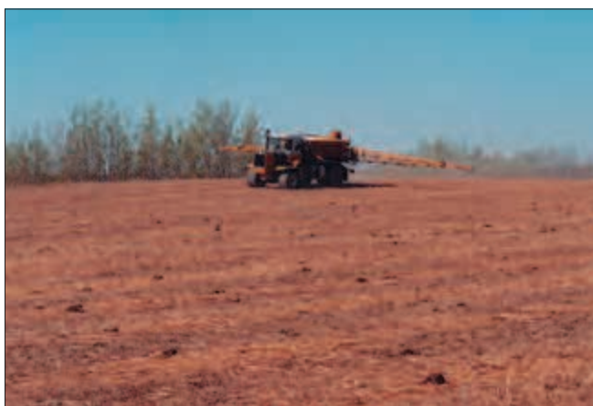
FIGURE 55 Commercial floaters provide even distribution of seed and fertilizer when overseeding pastures or broadcast seeding on cultivated land
