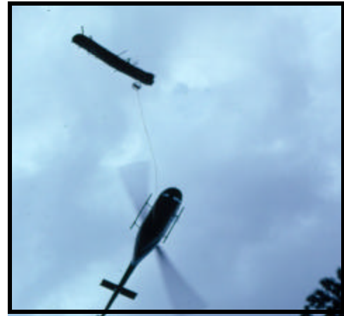
Helicopter long-lining beetle infested log to burn site.
