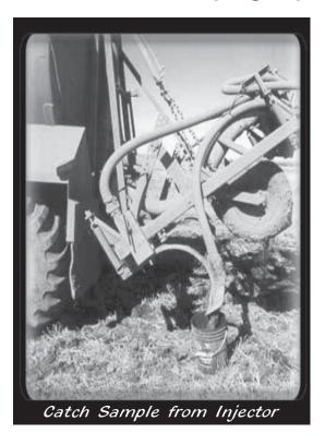
It is also possible to take manure samples directly from the manure application equipment. If a manure tanker is being used, single samples can be taken from each of several tanker loads, mixed and sub-sampled in order to obtain a representative sample. A clean, plastic pail should be used to collect the sample from the unloading port or the opening near the bottom of the tank.
