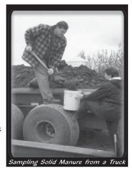
A well-mixed sample (approximately one litre) should be placed in a freezer bag or tightly sealed plastic container. The sample should be placed in an outer bag that can be sealed to prevent leaks and kept cool or frozen until transported to the lab for analysis.
