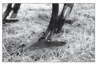
Figure 3. Sweep injector
