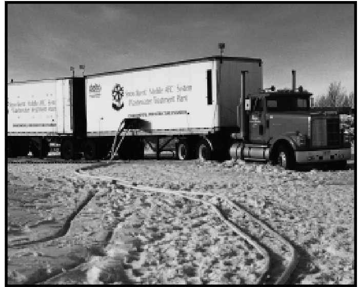
Delta Engineering Ltd.'s fully mobile Snowfluent AFC plant is mounted on a dual tractor-trailer rig, with an integrated power supply.
