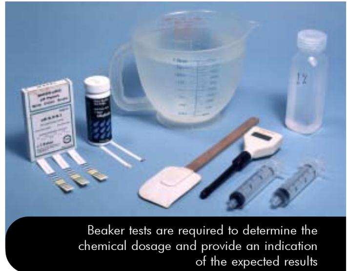
Beaker tests are required to determine the chemical dosage and provide an indication of the expected results
