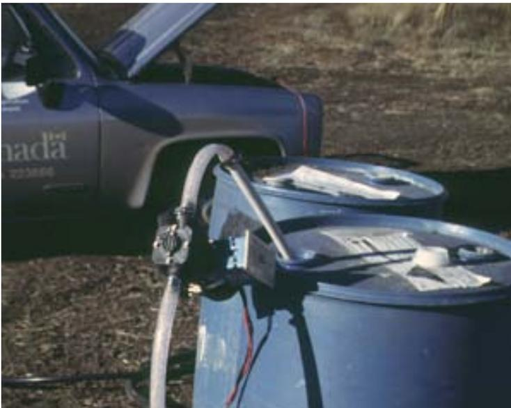
The coagulant chemical is pumped from the plastic barrel. Rinsing of the pump is critical to prevent impeller corrosion
