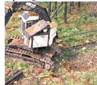
Tracks minimize the impact of machinery on soils by distributing the weight across a greater surface area.
