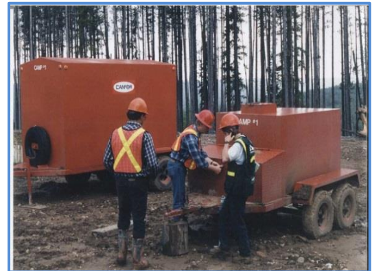
Figure 48 Fire Equipment Trailers
