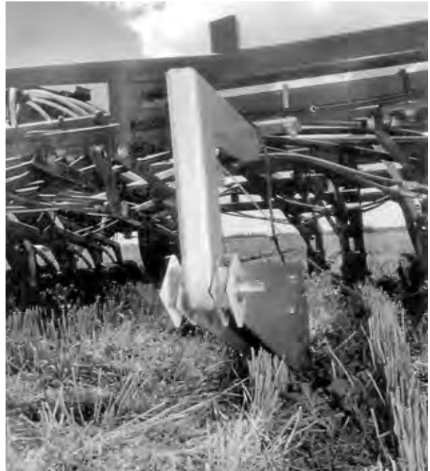
Figure 14. The Smart Hitch Guidance System mates to a steering mechanism on the cultivator. Photo Source: Western Producer/Michael Raine. Used by permission.
