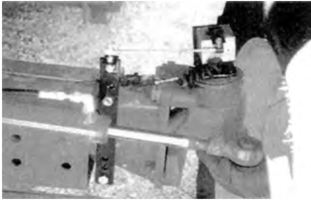
Figure 12. Tri-R Innovation System steering control - feedback sensor mounts onto steering axle. Photo Source: Company Literature
