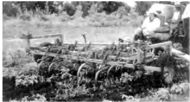
Figure 7. Operator Steered Cultivators are safer if the operator is positioned at the rear of the cultivator, facing direction of travel.
