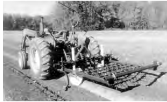
Figure 6. The Williams Tool System uses guide wheels as a way of manually guiding the cultivator. Market Farm Implement Catalogue photo, used by permission.
