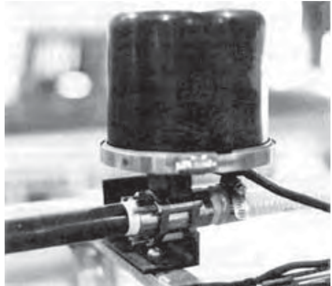
FIGURE 3. Motorized Control Valve.
