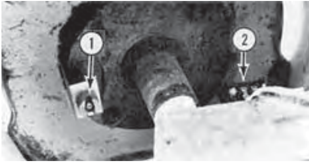
FIGURE 2. Wheel Transducer: (1) Magnet, (2) Detector Switch.
