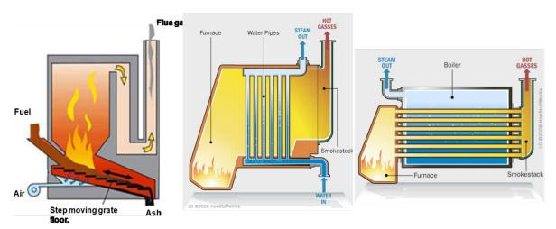
Figure 13: Left – grate furnace, centre – fire tube boiler (up to ~25MW), and right – water tube boiler (from ~2MW +). Furnace and boiler components combine to form what is normally referred to as a "boiler". Source: Natural Resources Canada and FVB Energy via Canadian District Energy Association *Biomass for District Heating* module.
