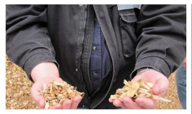
Figure 8: Different kinds of chip. To the left the smaller chip meets the European 'G30' standard and to the right the 'G50' standard. Source: Wood Waste 2 Rural Heat
