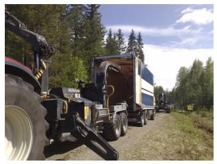
Figure 10: Roadside chipping operation in Finland using a farm tractor. Source: FPInnovations
