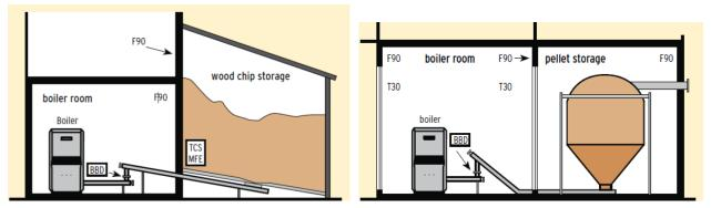
Figure 14: Examples of Austrian design of wood chip (up to 400kW) and wood pellet (up to 150kW) systems. F90 – an Austrian fire resistant wall specification, T30 - fire stop door spec, BBD – burn back safety device, TCS – temperature control device in fuel storage, MFE – manual fire extinguisher. Source: OÖ Energiesparverband. http://www.esv.or.at/english/home/
