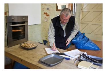
Figure 9: Measuring moisture content of woodchip using the oven dry method. Source: The Ashden Awards for Sustainable Energy (photo of Midlands Wood Fuel Ltd.)
