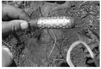
Figure 4. Watermark sensor by Irrometer.
