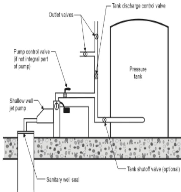
Figure 2. shallow well jet pump installation
