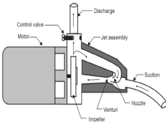
Figure 1. Shallow well jet pump operation.
