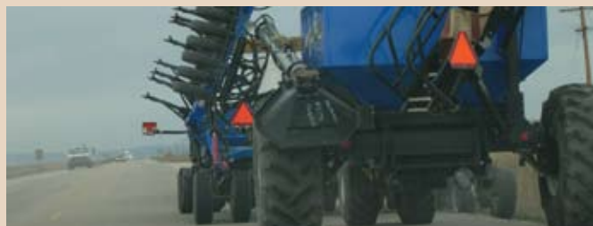
Make sure proper placards are in place when transporting equipment.
