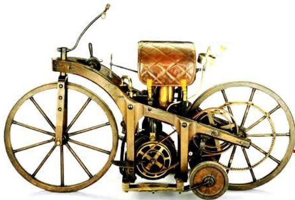
1885 – Daimler-Maybach motorcycle used a solid wooden structure
