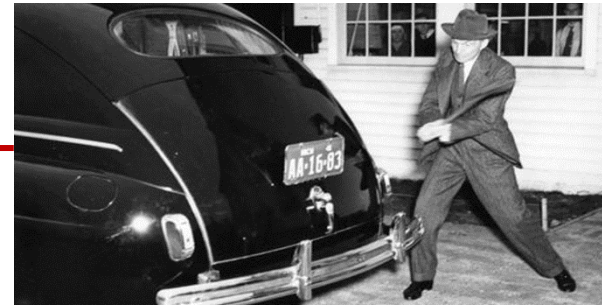
1941 - Ford Motor Company used hemp, ramie, wood flour and other NF in a phenol-formaldehyde resin
