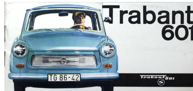
1962 – VEB Trabant used cotton waste in a phenol resin
